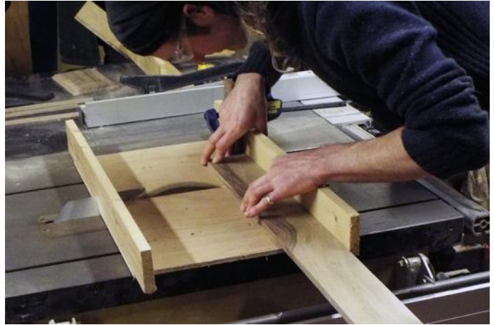
Cutting the sides of the box to length on the cross-cut sled
