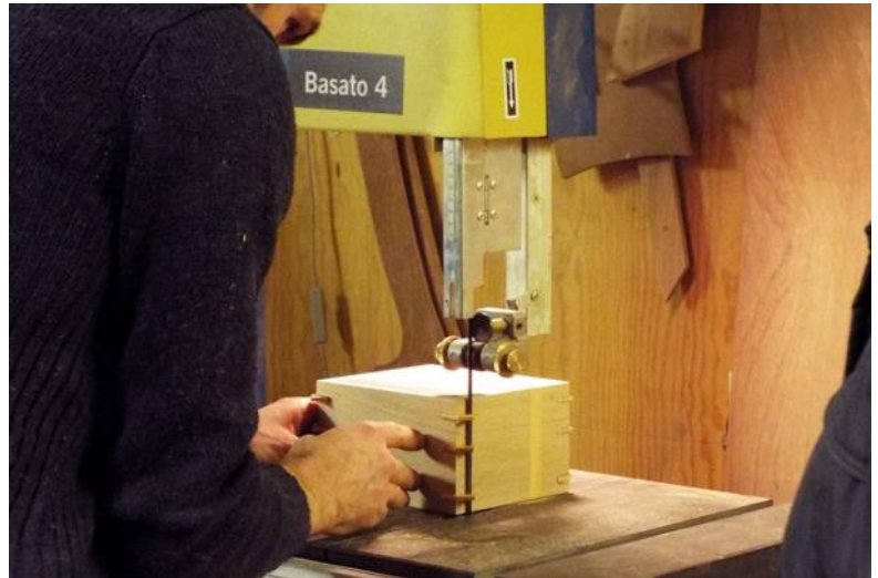
Trimming the keys on the bandsaw
