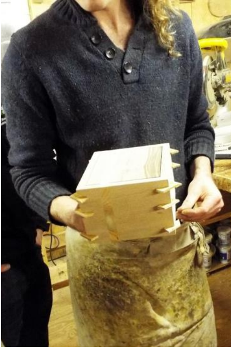
A semi-finished box with the rough corner keys
