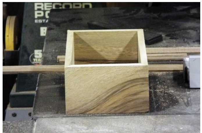
The box laid out with 45° miter corners
