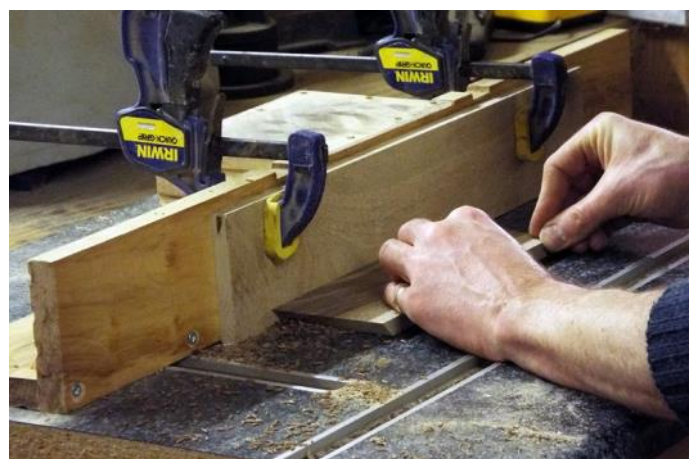
Preparing the sides of the box on the router table
